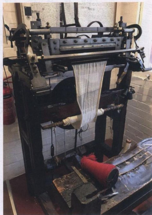
A narrow knitting frame, circa 1760. The frameworker could work one panel at a time. This machine still works and can make shawls. Photo courtesy of the Framework Knitters Museum, Ruddington.
